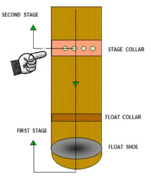
Two stage cementing is a technique where a tool called stage collar is placed in a casing string - this collar allows ports or holes to be opened and circulation can be performed through them.
